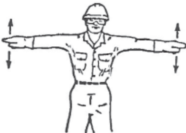
LEVEL: Arms extended, palms down, plane of arms indicates direction of movement.
